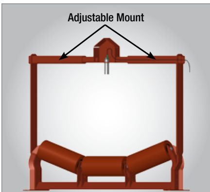
Fig 22.1 Adjustable Mount per Belt Width
